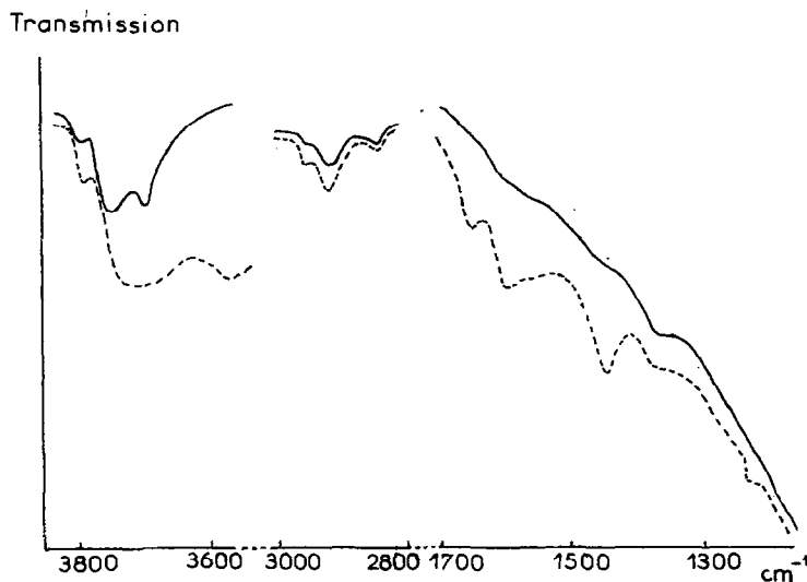
FIG. 2. Hydrogenation of an impure alumina sample: — initial sample --- after hydrogenation at 300°C (80 torr H 2 , 3 hr).
